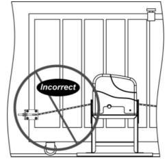
2). The opener must be parallel to the gate.
