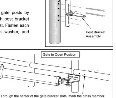
Through the center of the bracket slots, mark the fence post. Drill ¢ 10.5 holes in the
