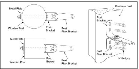
Both round and square post can be used because of the curved design of the post brackets. When mounting the post brackets, use bolts long enough to pass through the entire post. When mounting the post brackets to wooden posts, a larger-size washer or metal plate should be used between the bolts and the wooden post to ensure the stability of the fastening hardware when thrust is used.
