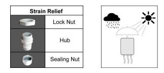
CAUTION: Install the Control Box in a well ventilated place protected against rain and sunlight. NOTE: It is strongly suggested that the control box should be mounted in the side of Master Gate (Gate 1), so that the electric lock can be installed correctly and work properly (See Page 9).
